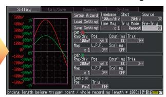
The help text crawls along the bottom of the screen, describing the function of the setting at the blinking cursor. The enhanced "Waveform Monitor" window with level meter display facilitates changes to settings by simultaneously displaying real-time input waveforms.
