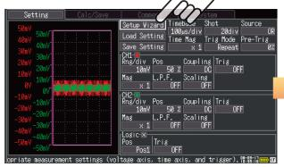
When powered on, the Settings screen appears along with the waveform monitor, and the new Setup Wizard blinks. By activating the Setup Wizard, you can easily navigate by following the simple instructions. Soon you will be operating the device like a seasoned professional.
