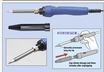
●2 stage heat switching system. ●Pulling the trigger boosts the output of normal position (Low) by 10 times. The pistol grip was designed through careful ergonomics research. It can be operated for extended periods comfortably even by someone with a small hand. The design allows full concentration on the work by making it easy to see the tip.
