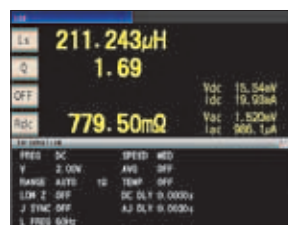
L, Q and Rdc continuous measurement screen
