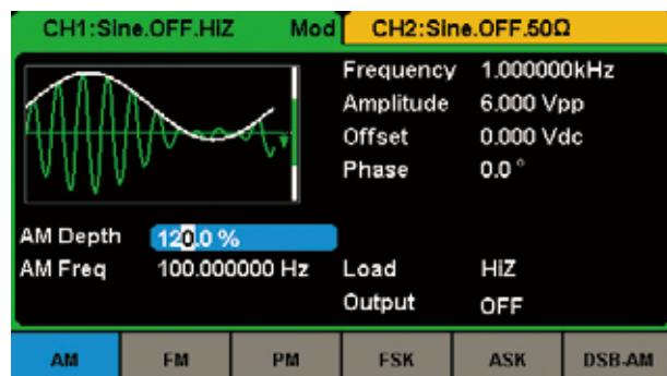
SDG2000X supports plenty of modulation types, such as AM、FM、PM、FSK、ASK、DSB-AM, and so on. The modulation source can be configured as "Internal" or "External".
