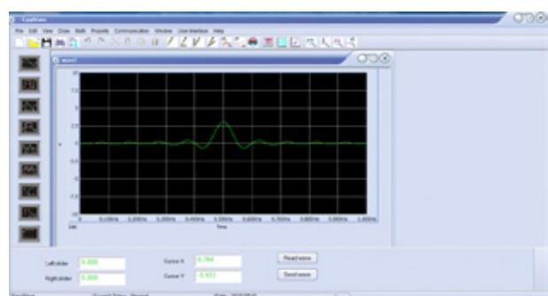
EasyWave is a powerful arbitrary waveform editing software that supports several ways to generate arbitrary waveform such as manual drawing, line-drawing, equation-drawing, coordinate-drawing, etc. It is quite convenient for users to edit their own arbitrary waveforms through EasyWave.
